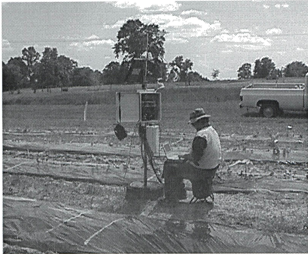
Fig. 2. Programable data acquisition system for monitoring soil, plant and air temperatures, light level and soil moisture content and tension.
